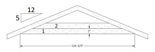
6. Studs in a framed wall are placed 16 inches apart. A sloped wall presents a challenge in that each stud must be cut to a different length. If the top plate has a slope of 10/12, set up a proportion to calculate the difference in length rounded to the nearest 16<sup>th</sup> of an inch.
