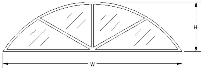
Find the radius of an arch window accurate to the 16<sup>th</sup> of an inch, which has a width of 42 inches and a height of 12 inches.
