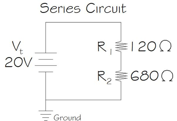
31. Use the Current Divider Formulas to calculate currents  $I_1$  and  $I_2$  at each resistor  $R_1$  and  $R_2$ .
