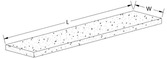
2. The volume (V) of concrete for a driveway or sidewalk is often estimated by  $V = \frac{LW}{80}$ .
